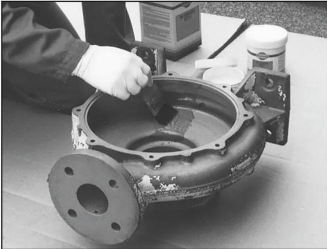
CERAMIC BRUSH ON is a highly advanced thixotropic liquid that contains highly abrasion resistant ceramic particles suspended within a high strength epoxy resin. This coating can be easily applied by brush to equipment to maximize service life by providing protection against abrasion, corrosion and chemical attack. Available as Red, Blue or White.
